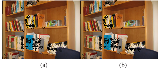
Figure 3. Reprojected points from the estimated localization. Image (a) shows the points projected when the camera is placed according to the (2,2) solver and (c) when the camera is located as the three point solver proposed.
