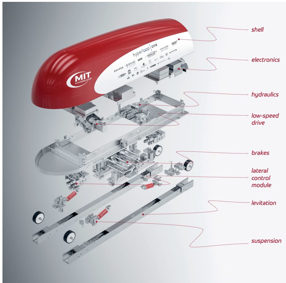
Figure 1. Exploded view of the MIT Hyperloop Design.
