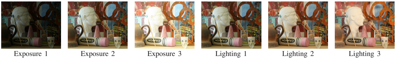
Fig. 12. The left image of the Art dataset with three different exposures and under three different light conditions. The right images have been captured under the same conditions, such that 3x3 combinations of matching are possible, separately for different exposures and light conditions.
