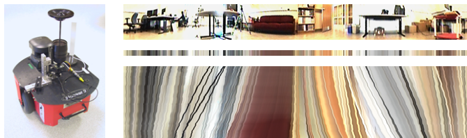
Fig. 1. Our robot with omnidirectional camera, a sample panoramic view, the circular 1D image formed by averaging the center scanlines of the panoramic view, and the epipolar plane image (EPI), a “stack” of one-dimensional images over time as the robot travels.
