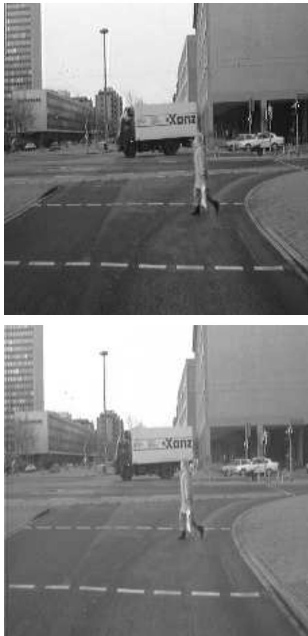
Fig. 5.3. The left and right images of the street pair used as test data for the gradient-based stereo method. The image pair is challenging in that it contains large untextured areas and global intensity differences due to different camera characteristics.
