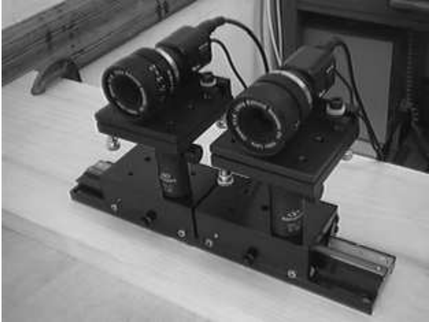
Fig. 1.9. A stereo rig with two identical, parallel cameras.
