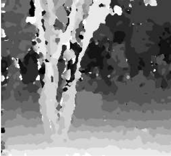
Fig. 5.8. Disparities for the tree image pair. Gray levels correspond to disparities: lighter is closer, darker is farther away.
