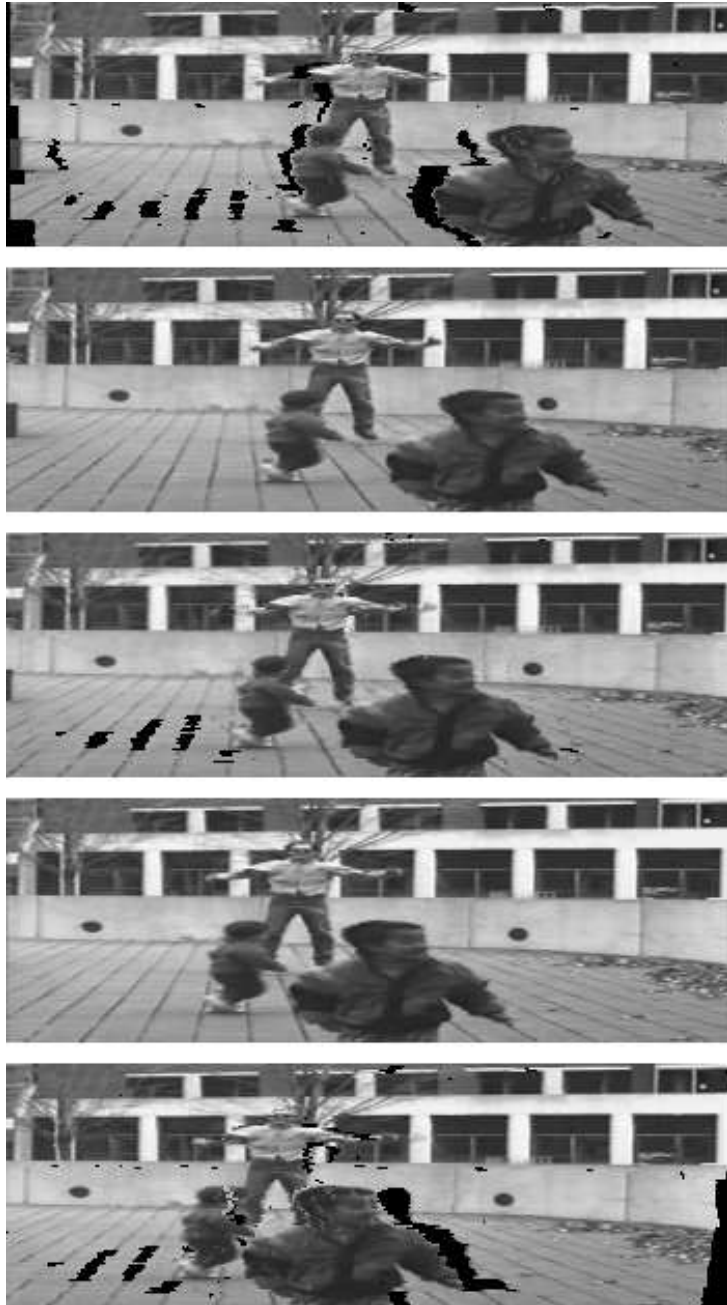
Fig. 3.5. Synthesized views for the kids image pair from different positions along the baseline. The second and fourth row contain the original images. The holes are shown in black.
